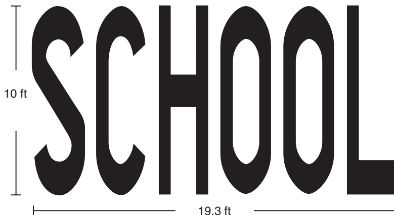
Figure 7C-1. Two-Lane Pavement Marking of “SCHOOL”
